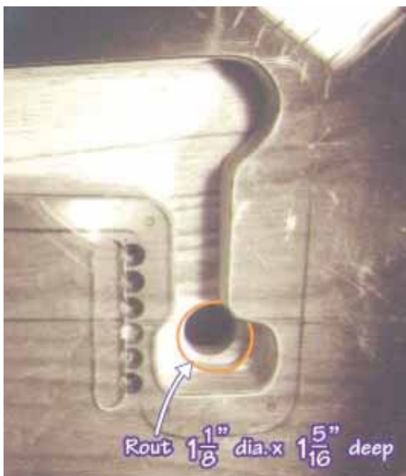
Photo H: Area for deeper routing
