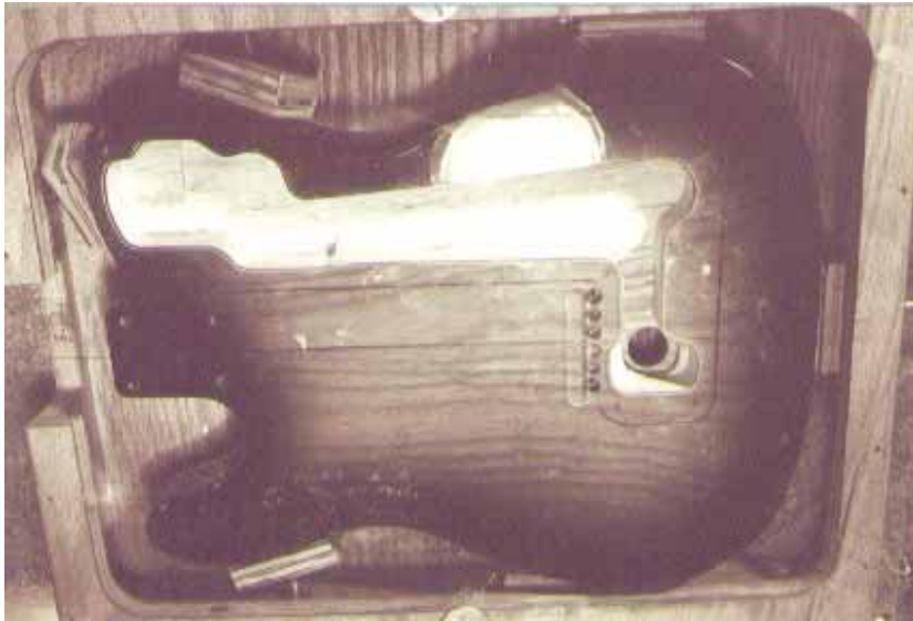
Photo F: Routing box and clear template ready for routing
